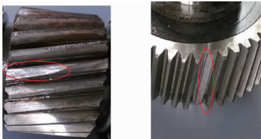
(a) 小齿轮齿局部断裂 (a) Pinion tooth partial fracture (b) 大齿轮断齿 (b) Gear tooth fracture
