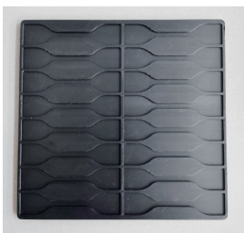
(a) 哑铃状试样模具 (a) Bar-shaped specimen mold
