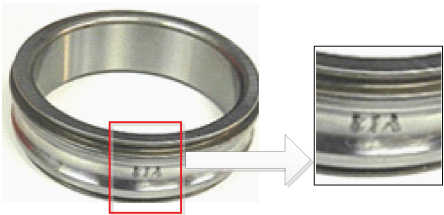
图 12 行星轴承内圈故障 Fig. 12 Planet bearing with inner race fault
