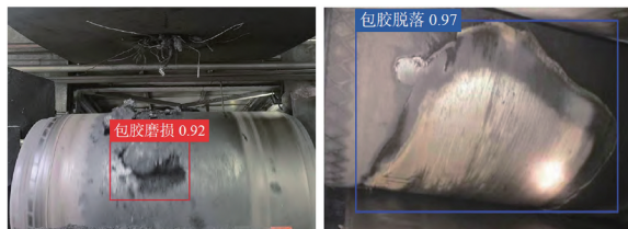
(c) 滚筒磨损与包胶脱落 (c) Roller wear and glue shedding
