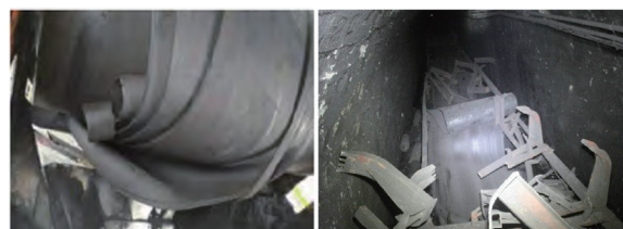
(a) 输送带纵向撕裂与断裂 (a) Longitudinal tearing and fracture of conveyor belt
