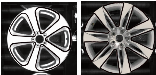
(b) A4、A5型号轮毂轮辐形状的匹配结果 (b) The spokes shape matching results of wheel A4, A5
