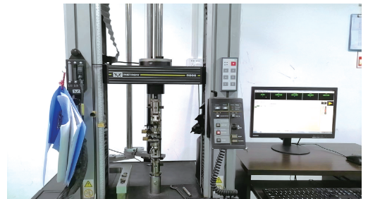
(a) Instron 5866 万能试验机 (a) Instron 5866 universal testing machine
