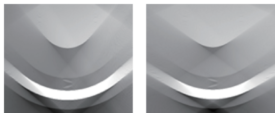
(a) 射线源距探测器170 mm (a) SOD=170 mm (b) 射线源距探测器270 mm (b) SOD=270 mm
