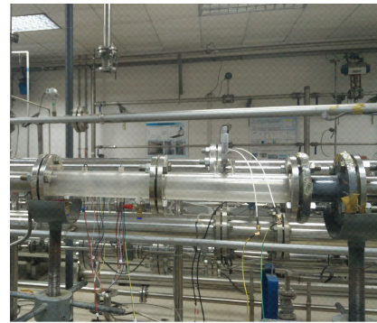
(b) 环状流液膜动态测量装置实物图 (b) Object picture of annular flow liquid film dynamic measuring device
