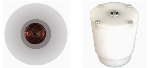
(a) 针式 EMAT 线圈 (a) Pin-type EMAT and coil (b) 针式 EMAT (b) Pin-type EMAT
