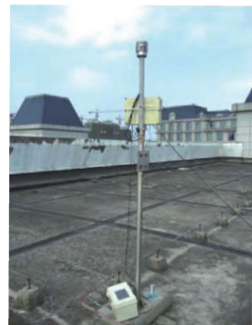
(b) 三维大气电场仪测量实验 (b) Three-dimensional atmospheric electric field instrument measurement experiment
