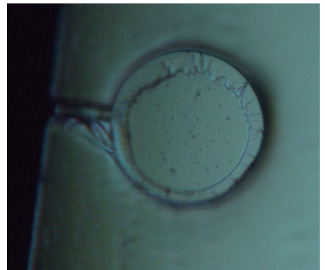
图 3 经过蒸发 Al 电极和解理后的器件显微图像 Fig. 3 Microscopic image of the device after evaporation of Al electrode and cleavage
