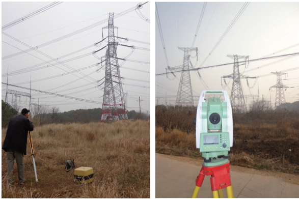
(c) 全站仪横线路测量 (c) Measurement from the direction of horizontal line by total station instrument (d) 全站仪顺线路测量 (d) Measurement from line direction by total station instrument
