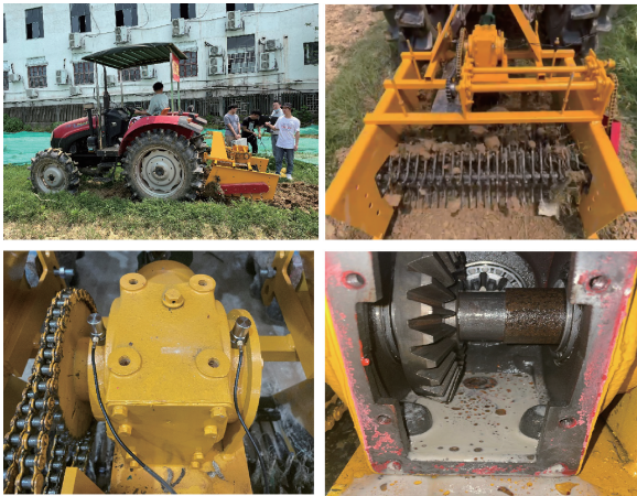
图 13 蒜头收获机齿轮箱故障诊断实验 Fig. 13 Fault diagnosis experiment for gear box of chinese onion harvester
