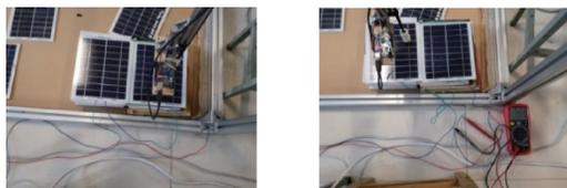
(a) 串联 (a) Series (b) 并联 (b) Parallel
