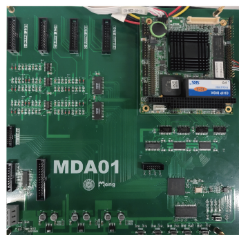
(b) 多通道数据采集系统及实时控制计算机 (b) Multi-channel data acquisition system and real-time control computer
