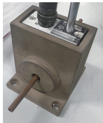
(c) NTSL-F型穿过式涡流检测探头 (c) NTSL-F through-type eddy current testing probe
