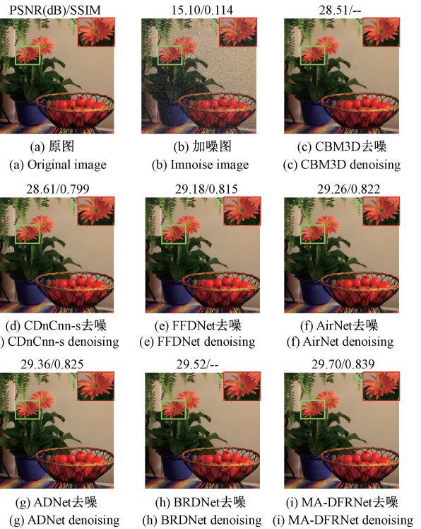
图6 不同网络在 McMaster 里图像的去噪结果( \sigma = 50 ) Fig. 6 Denoising results of image in McMaster with different networks ( \sigma = 50 )
