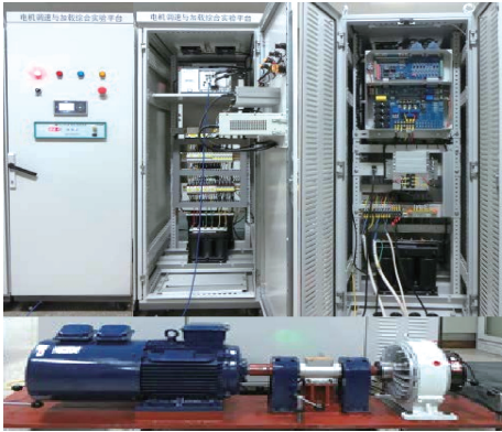
图 7 电机调速与加载综合实验平台实物 Fig. 7 Physical maps of a comprehensive experimental platform for motor speed regulation and loading
