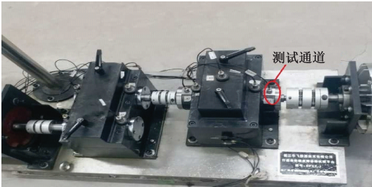
图 4 行星齿轮箱实验台现场测点布置图 Fig. 4 Layout of measuring points on the planet gearbox test platform
