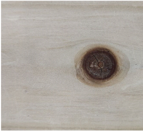
图 7 带有节子和裂纹缺陷的木材试样 Fig. 7 Wood sample with crack and knot defects
