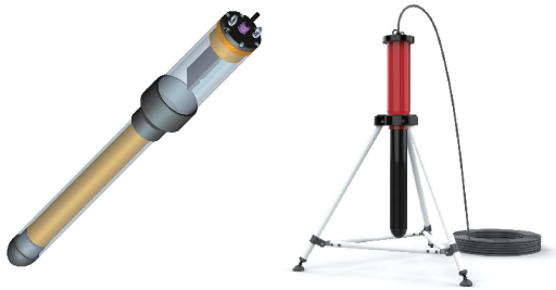
图 3 AETA 电磁扰动传感探头结构和实物 Fig. 3 Structure and physical diagram of AETA electromagnetic disturbance sensing probe
