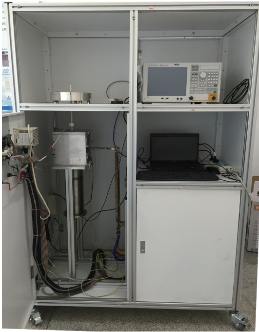
图 5 圆柱腔复介电常数变温测试系统实物 Fig. 5 Picture of the cylindrical cavity complex permittivity variable-temperature measurement system
