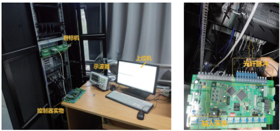
(a) 半实物仿真系统组成 (a) Physical composition of hardware-in-loop simulation (b) 控制器实物连接图 (b) Physical connection of controller
