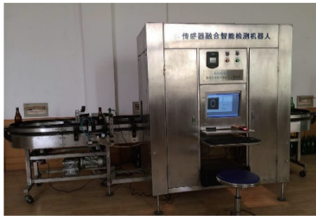
(a) 空瓶检测系统实物 (a) Photo of bottle detection system
