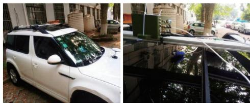
(a) 双天线RTK安装图 (a) Installation drawing of dual antenna RTK
